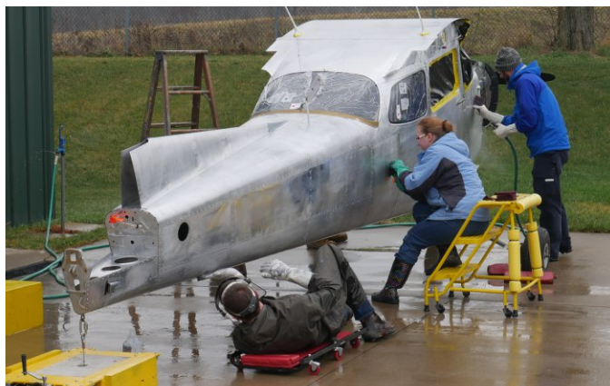
Aaron works with Chuck and Jenny to prepare MAG's Cessna 172 for paint.
