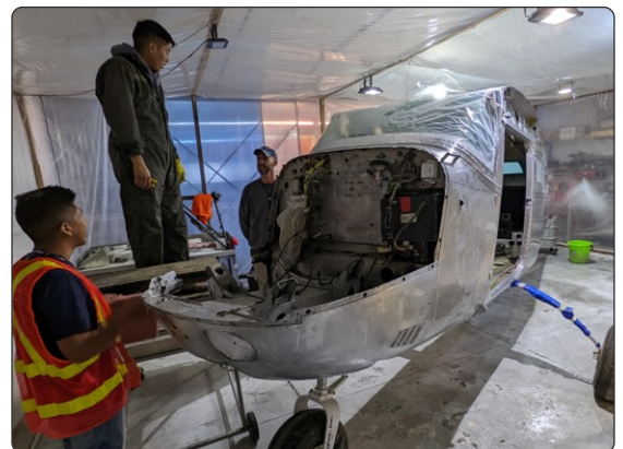
Preparing the 206 fuselage for paint.
