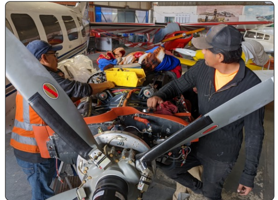
Some of the Bolivian mechanics finishing the engine installation on the Navajo.
